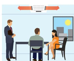
Indirect air flow by detecting movement
