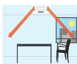
Circulation by Detecting no movement (10min.)
